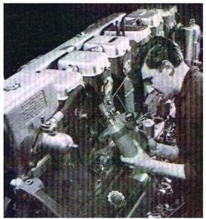
Purolator filters connected by Lockheed Avery hoses are fitted on Gardner engines for fuel and lubricating oil filtration
